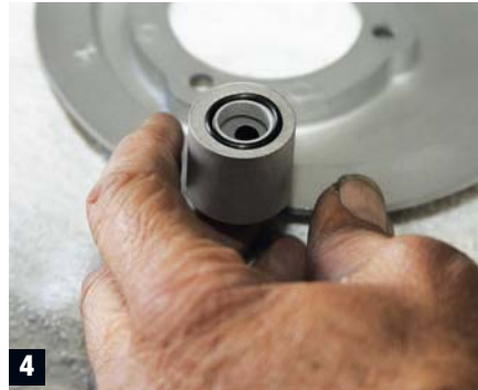
Next, new O-ring breather gaskets were placed onto the Ness backing plate, along with a new EFI gasket. A small dab of 575 sealant kept them in place 'til the backing plate was tightened down.
