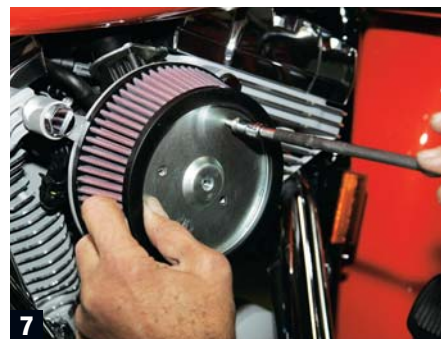
Then the Ness Big Sucker air filter was installed with the stock air-filter cover. ▶
